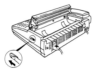
2. Place a new paper roll in the compartment. Be sure the paper exits from the top of the roll as shown.
